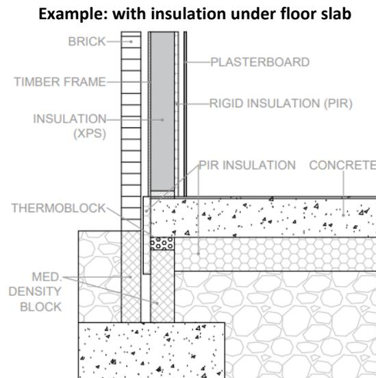
**Specification to eliminate or reduce thermal bridge at the junction of a timber frame wall with a suspended floor**
